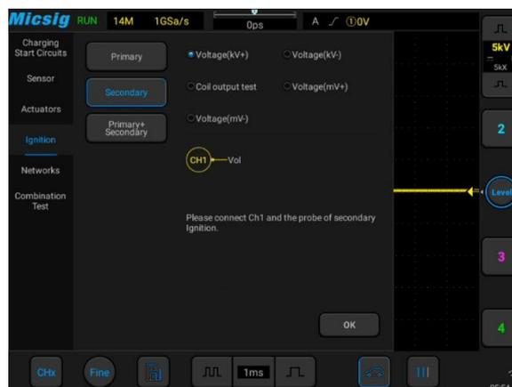
▲ The ignition system of a car is usually composed of primary and secondary coils and spark plugs. SATO can test both Primary and Secondary ignition signals, to find out possible malfunction.
