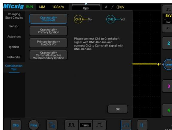
▲ The electronic faults can be complicated, use SATO to perform combination tests, by comparing the collected various waveforms, it helps users judge faults by analyzing the timing and quantitative relationships between waveforms.
