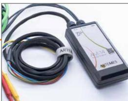
power logger for measuring energy consumption
