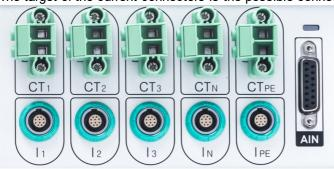
The current can be connected either directly (screw terminals) or with a sensor (Lemo connector).
