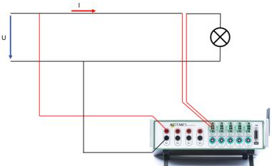
It is recommended, but not necessary to use fuses of type 500mA for the voltage connections.
