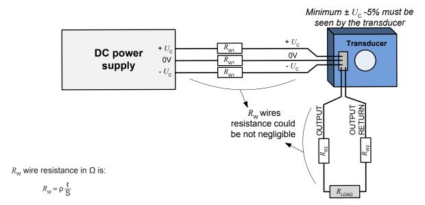
S: Cross section of wire in m<sup>2</sup>
