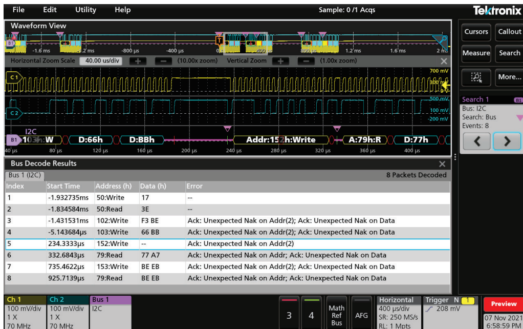
A bus waveform provides time-correlated decoded packets while the bus decode table presents all the packets from the entire acquisition; search can be used to navigate
